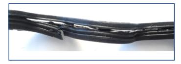
It should be considered that the tightness of these type of gasket usually is between 8-12Nm, and if the screws are tightened without using a dynamometer, it's probable that its reaching the 25Nm easily without realizing it.
