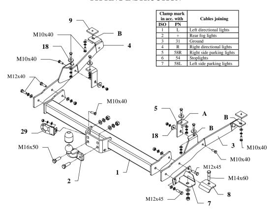
This towing hitch is designed to assembly in following cars: **FIAT DUCATO, PEUGEOT BOXER, CITROEN JUMPER, 2WD and 4WD, metal build-up, loading platform,** produced since 05.1994 till 06.1999, catalogue number **R08** and is prepared to tow trailers max total weight **2000 kg** and max vertical load **100 kg**.
