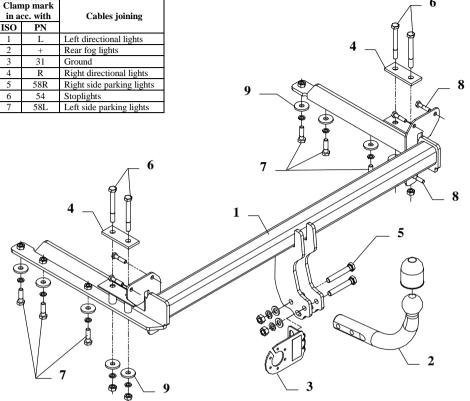
This towbar is designed to assembly in following cars: **KIA SEPHIA II, KIA SHUMA II,** produced since 1998 till 04.2001, catalogue no. **T06** and is prepared to tow trailers max total weight **1350 kg** and max vertical load **50 kg**.
