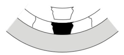
Close to the bond line the vertical cracks run.
